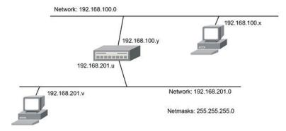
In this picture, assume that the computer at 192.168.100.x wants to send something to a computer at 192.168.201.v. The mask calculation creates a comparison of 192.168.100.0 versus 192.168.201.0, which shows that the network portions don't agree, and that the traffic has to be routed.
