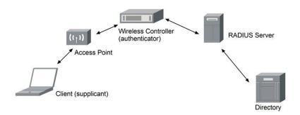
Because the access level granted can be based on the response from the directory, we can have a single authentication process and a single SSID shared by staff and students. Each person or group can be assigned a separate role and VLAN as a function of their AD group memberships or ability to authenticate.
