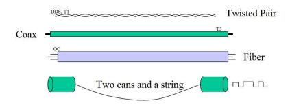
Network interfaces modulate data across the physical layer using electrical signals, pulses of light or radio, depending on the transmission ability of the medium. For two cans and a string, it would be vibrations.<sup>1</sup>
